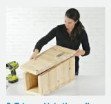
5. Trim and join the walls. Following cutlines, trim the walls with a circular saw. Lay down a back wall and run glue along the long edges; add two side walls on edge. Glue a front wall on top. Drill pilot holes on the front and back wall edges; secure with 2½-inch screws.
