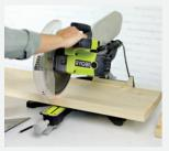
1. Cut the parts to length. Download the cut list from www.house.one. Using a miter saw, cut the seat, stringer, and legs. Then cut the seat's two trim pieces.
