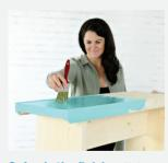
8. Apply the finish. Fill the screw holes with exteriorgrade wood filler. Sand the assembly smooth. Apply one coat of exterior solid stain, let dry, and repeat. Place the finished bench amid greenery, and prepare to take a seat.
