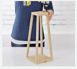
2. Assemble the lantern frame. Drill pilot holes through the top and bottom pieces and into the square dowels. Secure the dowels with wood glue and screws.
