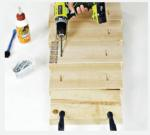
3. Join the boards. With the bottom board clamped to your worktable, glue the boards' adjoining edges to create the four walls. Then use a drill/driver and 2½-inch pocket hole screws to attach the boards for each wall.
