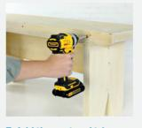
7. Add the seat and trim. Spread wood glue on the tops of the legs and center the seat on top. Glue on the front and back trim pieces flush with the top of the seat. Distribute three pilot holes along the length of each trim piece; fasten with 2-inch deck screws.
