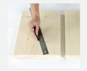
2. Mark a decorative notch in each leg. Draw a centerline 51/2 inches up from the bottom, and mark 4 inches in from each side. Connect the lines for a triangle cutout.
