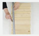
4. Draw cutlines. On the front and back walls, mark the width of the bottom boards at 9 inches (centered), then draw a line to the top corners. Mark the side pieces 7 inches wide at the bottom and 2 inches narrower at the top (centered) to fit inside the front and back walls.
