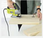
3. Cut out the leg notches. With the pencil lines as a guide, use a jigsaw to cut out the decorative notch in each of the leg pieces.
