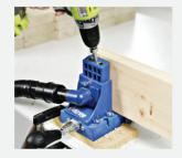
2. Drill the pocket holes. Line up the boards for each wall, from longest to shortest. Using a pocket hole jig, drill two pocket holes a few inches in from each end on one side of the four longest boards for each wall of the planter.
