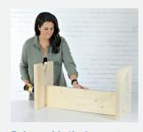
5. Assemble the base. Place the stretcher on edge and center it between the legs, cut edge flush with the work surface and the tops of the legs. Make two pilot holes in the face of each leg and drive 3-inch deck screws through them to secure the stretcher.
