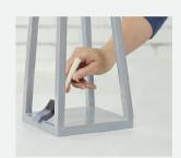
4. Sand the parts and apply your finish. Wipe on a coat of stain and let set for 2 to 3 minutes. Wipe away excess stain, let dry, then seal with a coat of polyurethane. Spray the hardware cloth with two coats of flat black spray paint.
